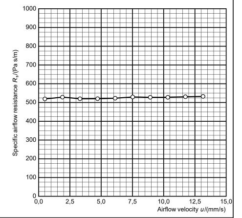
Specific airflow resistance  $R_s(0.5 \text{ mm/s}) = 518 \text{ Pa s/m}$
