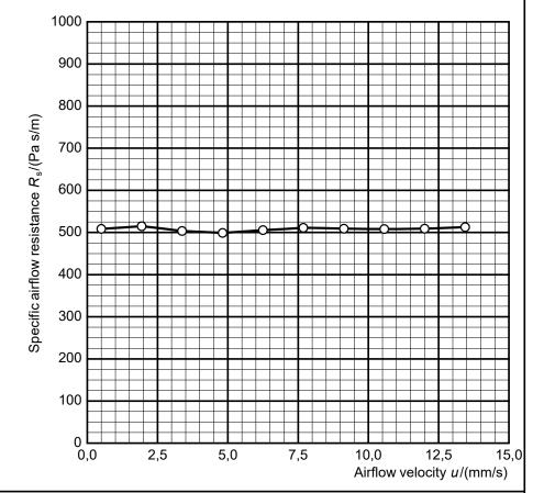
Specific airflow resistance  $R_s(0.5 \text{ mm/s}) = 501 \text{ Pa s/m}$
