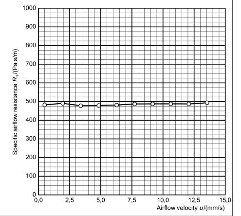
Specific airflow resistance  $R_s(0.5 \text{ mm/s}) = 475 \text{ Pa s/m}$
