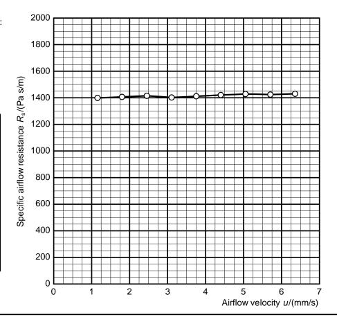
Specific airflow resistance  $R_s(0.5 \text{ mm/s}) = 1396 \text{ Pa s/m}$
